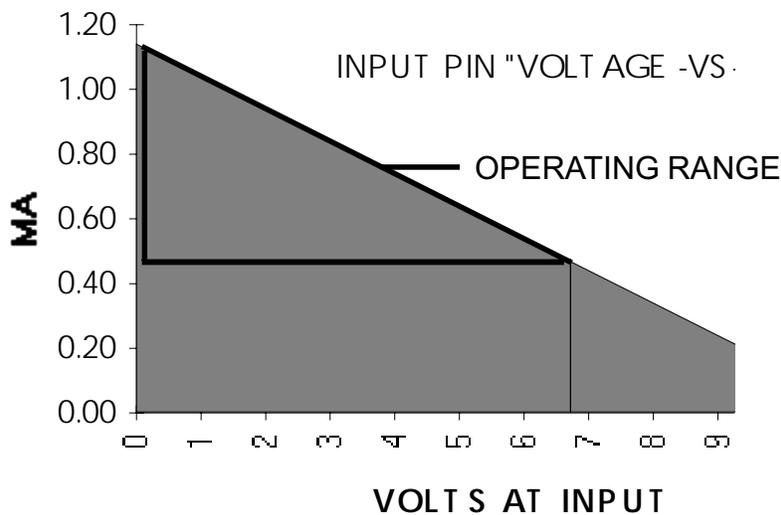
The minimum resistance to ground to produce an active COR is 7.5k or at least 0.5 mA is required.
