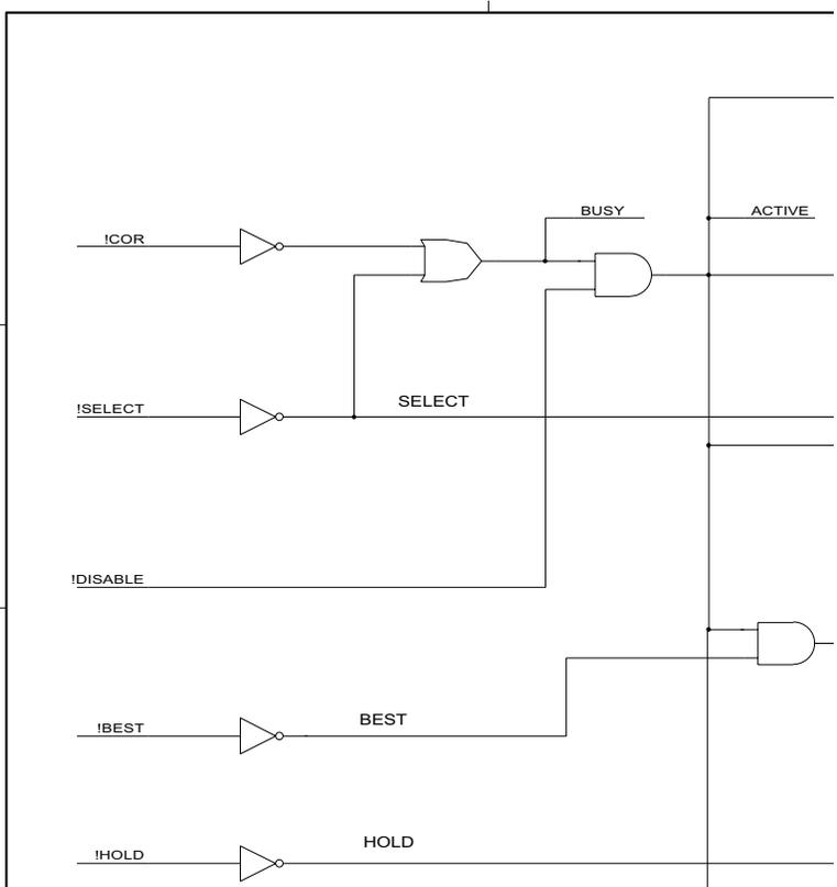
LOGIC EQUIVALENT DIAGRAM OF U15-U18
